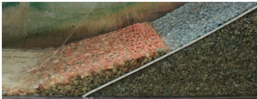
Fig. 14. Laboratory testing of a rockfill toe berm protection under through-flow conditions.
